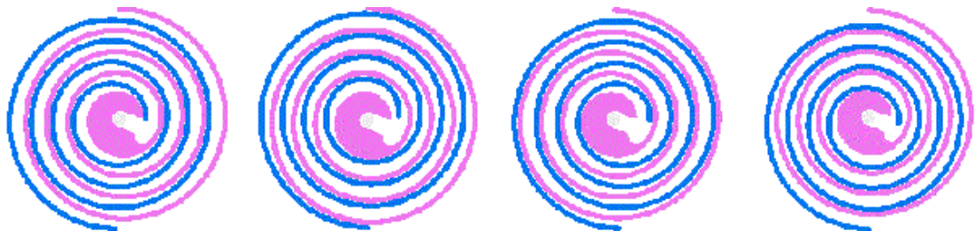
Fig. 2 Working principle of the Scroll pump
